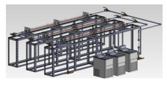
A heat exchange system with multistage heat storage containers filled with phase change materials having different melting points is experimentally investigated to develop a cascaded heat storage system that allows the use of low-level thermal energy in an ambient temperature range. (Image: Heat exchange system with multistage latent heat storage)
