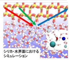
exist at the interface, It is clarifying whether it causes interface phenomenon. We are studying interface phenomena by molecular dynamics simulation and electronic state calculation at the buried interface. In particular, by comparing with experiments such as spectroscopy, we aim to elucidate the microscopic and molecular mechanisms at various interfaces such as inorganic materials, metals and biological systems.
