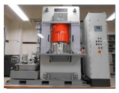
equipment which can realize such environment. We have succeeded in synthesis of novel rare-earth borides such as  $GdB_{12}$  and  $SmB_{12}$  which cannot be produced up to date. At present we are challenging the high-pressure synthesis of other lighter rare earth borides and new organic compounds.
